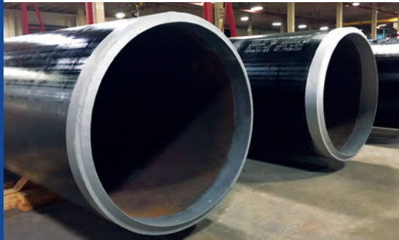
CARBON PIPE 36" 1.5" WALL
